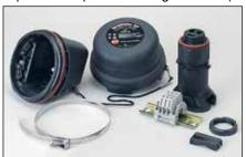
Terminator DP is designed to fabricate power connections, in-line/T-splice connections or for making end terminations. Electrical connections are made in terminal blocks utilizing nickel-plated copper terminals to ensure corrosion-free electrical integrity. The up front positioning of the terminal block permits easy access during assembly and for future routine maintenance.
