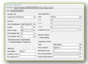
The Heater Information tab contains the variables that define a connection. Pipe type, exposure or max product temperatures, and heater types are examples of connection level variables.
